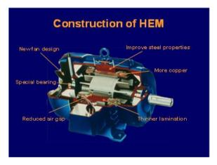
Standard motor is a compromise between efficiency, endurance, starting torque, and initial cost (with strong emphasis on the initial cost). Standard motor generally competes on price, not efficiency on the contrary. EEM competes on efficiency. not price.
